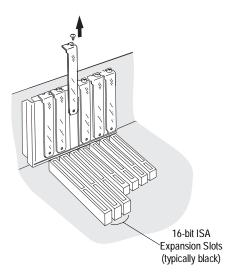
**Step 3:** Insert the host adapter in the slot; press down firmly so that the bus contacts are securely seated in the slot. If you are installing the AVA-1505AE secure it with the screw you removed in Step 2.
