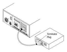
**Step 6:** Connect the SCSI device to a power source.
