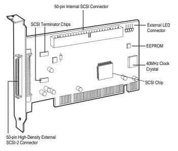
With the Adaptec software drivers, you can use AHA-2910C host adapters in computers running DOS/Windows $^{\mathbb{B}}$ , OS/2, Windows $^{\mathbb{B}}$ 95, Windows NT $^{\text{TM}}$ , UNIX, and NetWare.
