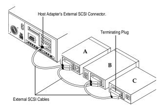
**Step 1:** Plug one end of the 50-pin high-density external SCSI cable into the host adapter's external SCSI connector.
