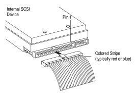
**Step 4:** Attach the remaining devices using the remaining connectors. These devices should not be terminated.
