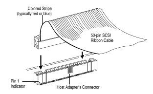
**Step 2:** Plug the internal SCSI cable into the host adapter's connector.
