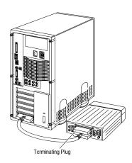
**Step 2:** To connect additional external SCSI devices, daisy-chain each device to the previous device until all devices are connected to each other. (The device at the end of the chain must have a terminating plug or have the on-board terminator enabled.) You need a 50-pin high-density external SCSI cable to connect external devices to the host adapter.
