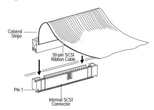
**Step 4:** Plug the other end of the 50-pin internal SCSI cable into one of the connectors on the last internal SCSI device in the chain. (This device must be terminated.) Make sure the colored stripe on the side of the cable is aligned with pin-1 of the SCSI device's connector.
