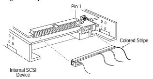
**Step 5:** Plug the remaining cable connectors into any remaining internal devices. (These devices must *not* be terminated.)
