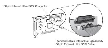
Secure the mounting bracket of the cable to the exposed card slot opening in the chassis of the computer.
