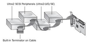
Internal Ultra2 SCSI peripherals come from the factory with termination disabled and cannot be changed. Proper termination is provided by the built-in terminator at the end of the Ultra2 internal SCSI cable provided in the kit.
