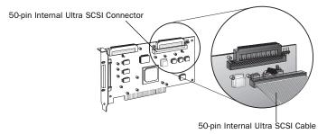
Plug the other end of the cable to a terminated Fast/Ultra Narrow SCSI peripheral.
