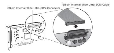
Plug the other end of the cable to a terminated Fast/Wide Ultra SCSI peripheral.
