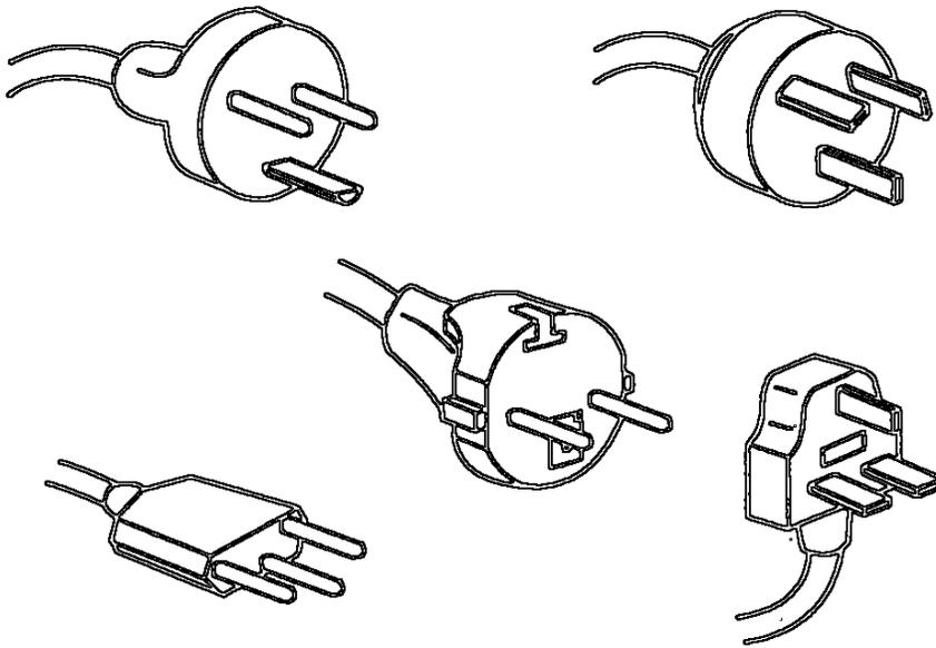
Figure 2-9 AC Power Cord Plug Ends
