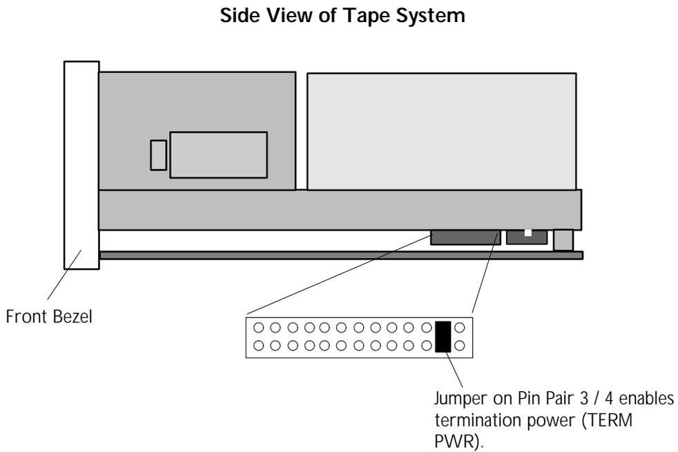
*Figure 2-2 Jumper Installed on Pin Pair 3 / 4 Enables Termination Power (TERM PWR)*
