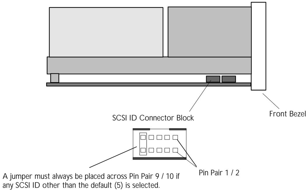
*Figure 2-1 Location of SCSI ID Connector Block*
