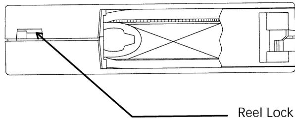
Figure F-1 Location of One of the Two Reel Lock Tabs on the DLTape
