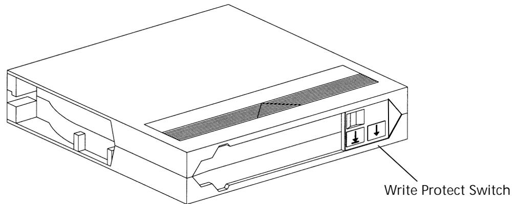
*Figure F-5 Location of Write Protect Switch*
