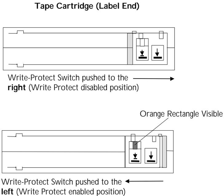
Figure 2-11 Write-Protect Switch on Tape Cartridge
