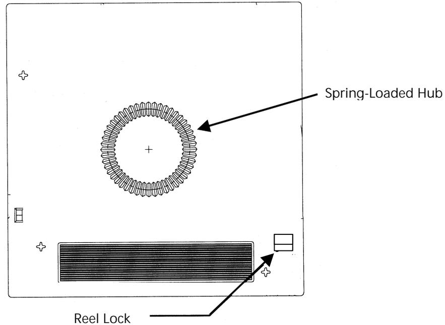
Figure F-2 Location of Reel Lock Opening and Spring-Loaded Hub on Bottom of DLTtape Cartridge
