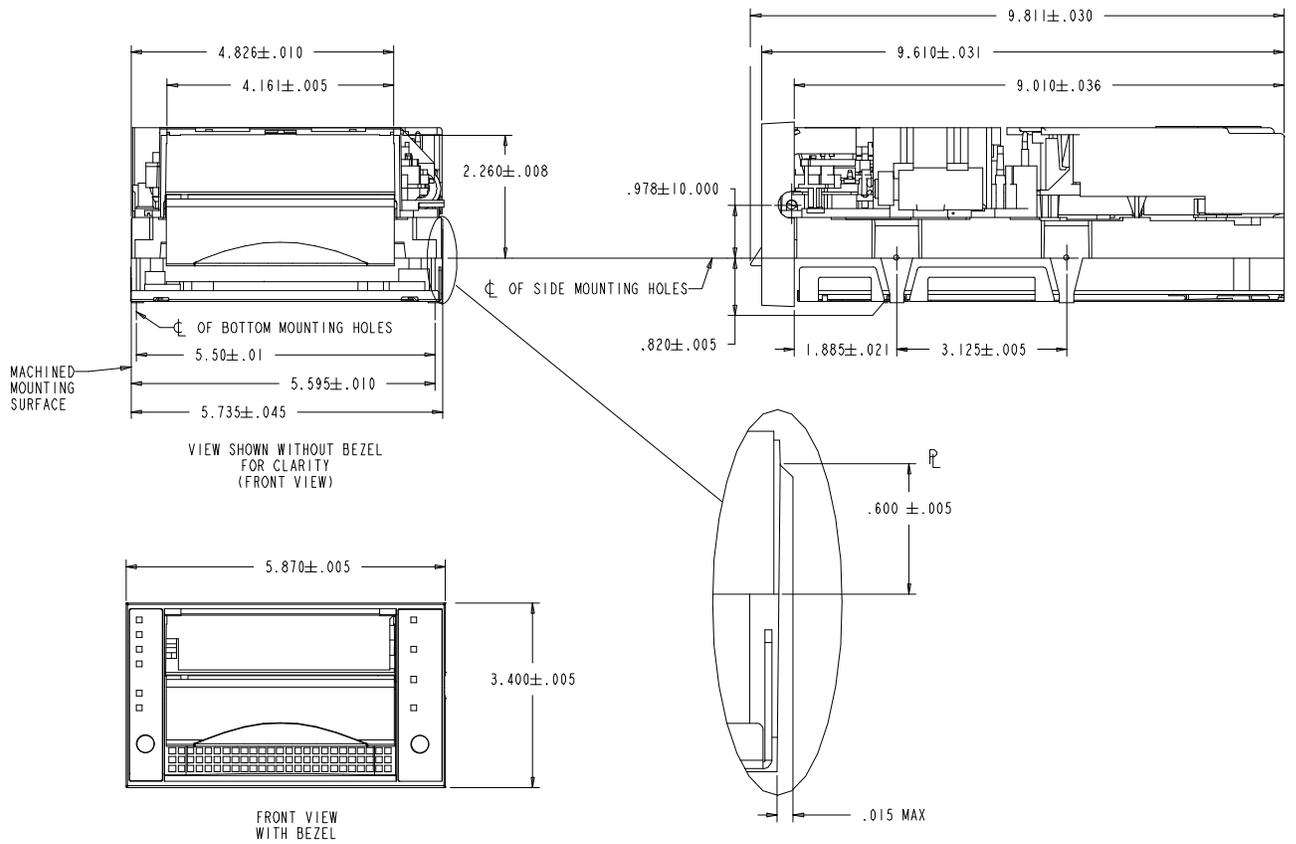
Figure 2-4 Locations and Dimensions for Mounting Holes
