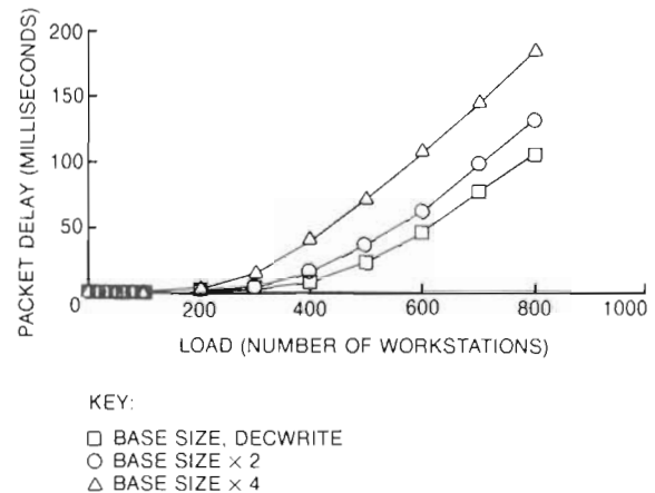
Figure 9 Varying Client Packet Size — Average Packet Delay versus Load
