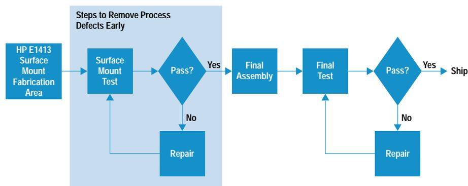
**Fig. 1.** The HP E1413 assemblies pass through a two-stage test and repair process. The surface mount test stage is aimed at detecting process defects and the final test stage is intended for calibration and performance verification.
