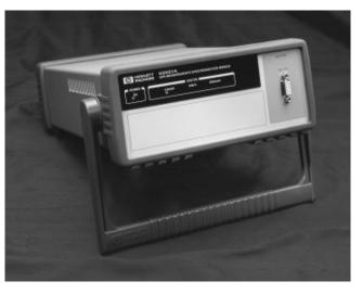
Fig. 7. HP 59551A GPS measurements synchronization module.
