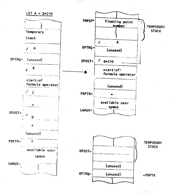
All operands (checked words) are addresses (i.e., C represents a pointer to the value of the simple variable C). Bits 7 - Ø of an operator entry contain the operators identifying code (See 'Basic Operators' Table) while bits 15-8 contain the operator's priority. Note the alternate-word structure of the stacks. The temporary stack holds intermediate values during the formula evaluation.
