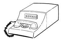
If your equipment is in two pieces, like this you have a regular telephone and a coupler/modem.
