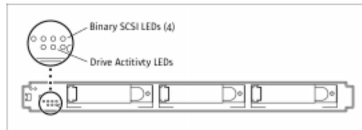
Figure 4. Front Panel Disk Drive LEDs
