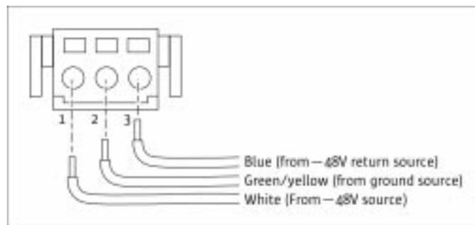
Figure 9. DC input power cables
