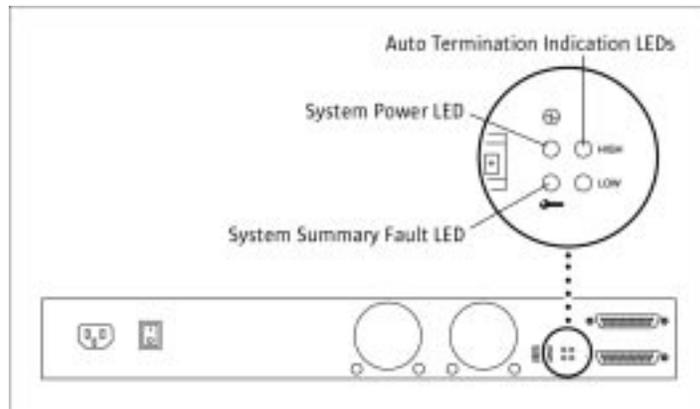
Figure 7. Rear Panel LEDs
