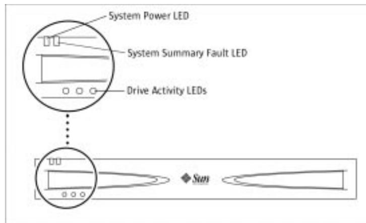
Figure 3. Front Panel System Power/Fault Indicators
