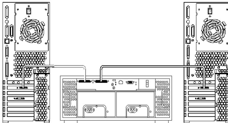
Figure 10. Sun StorEdge A1000 array connected to two hosts
