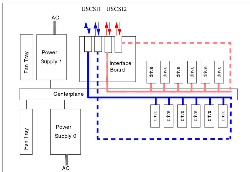
Figure 3. Sun StorEdge D1000 array system architecture
