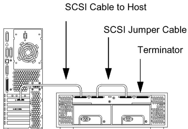
Figure 11. Bridged Sun StorEdge D1000 Array connected to single host
