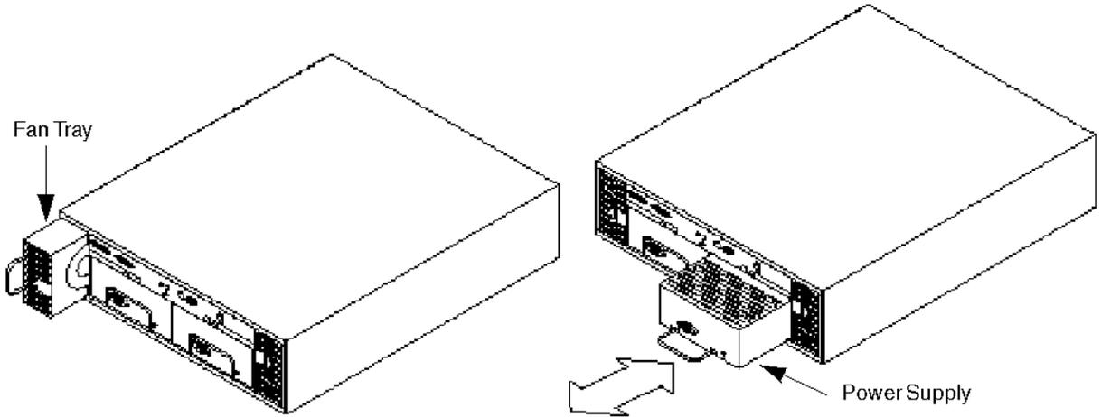
Figure 5. Sun StorEdge A1000 and D1000 arrays fan trays and power supplies
