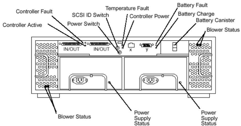
Figure 7. Sun StorEdge A1000 array rear view
