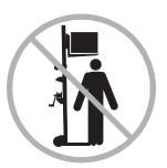
Use common sense and planning when transporting the machine on an incline, slope or stairs.
