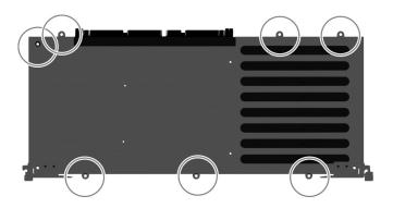
3. Using a Phillips No 2. screwdriver, remove the two flat head Phillips screws securing the plastic cover to the CPU/Memory board.
