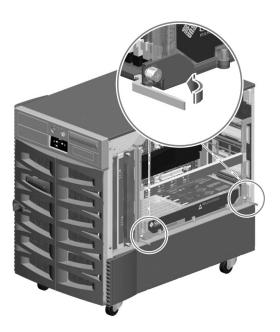
5. Hand-tighten the two captive screws on the CPU/Memory board.
