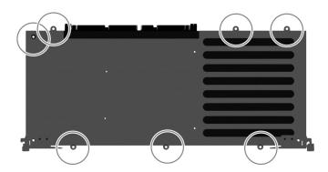
14. Using a Phillips No. 2 screwdriver, replace the two flat head Phillips screws that secure the plastic cover to the CPU/Memory board. Fully tighten the screws.
